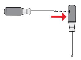
Seat the 6-lobe driver in the head of the screw and 2 apply firm downward pressure, while turning with the other driver to loosen the screw.
